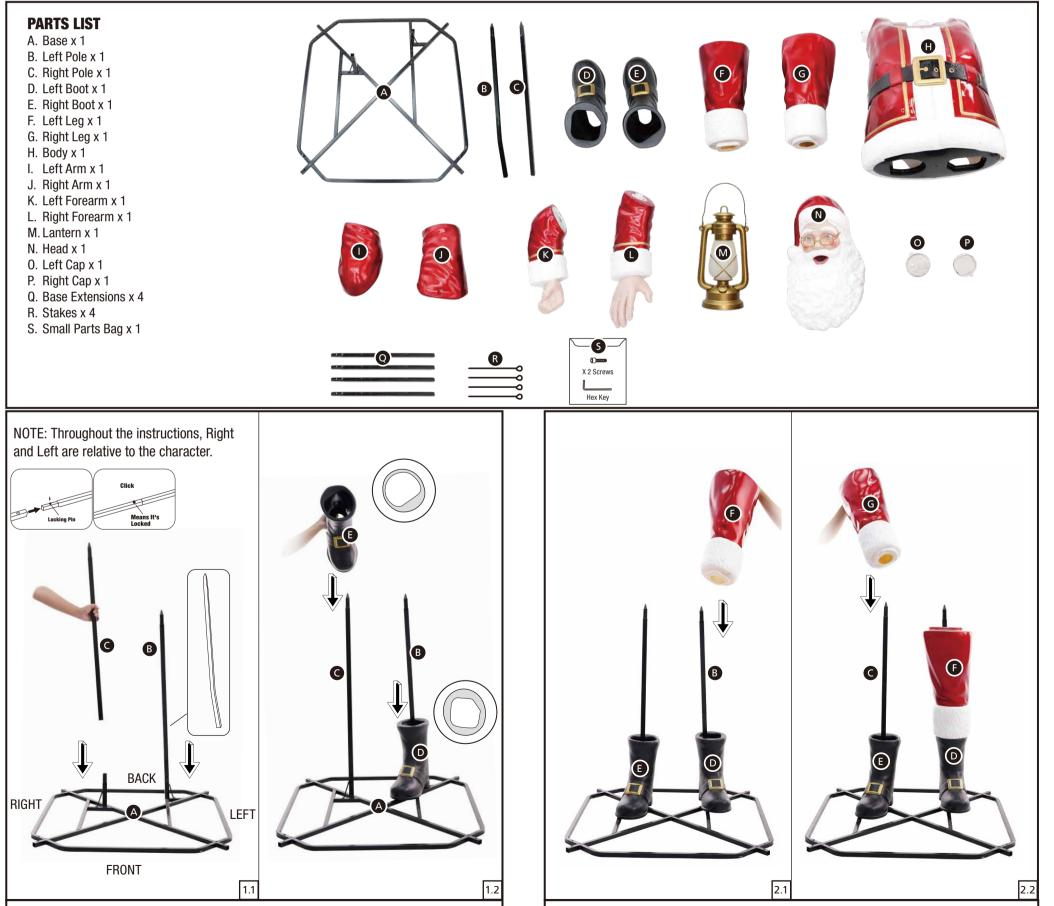
Attach the (B) Left Pole and the (C) Right Pole to their corresponding positions on the (A) Base using the quick connect push buttons and pre-drilled holes as shown in Figure 1.1. Then slide the (D) Left Boot over the (B) Left Pole and have it rest on the (A) Base. Slide the (E) Right Boot over the (C) Right Pole and have it rest on the (A) Base as shown in Figure 1.2.
