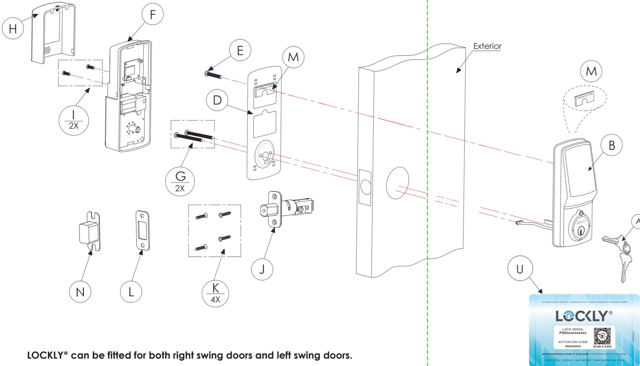
LOCKLY® can be fitted for both right swing doors and left swing doors.
