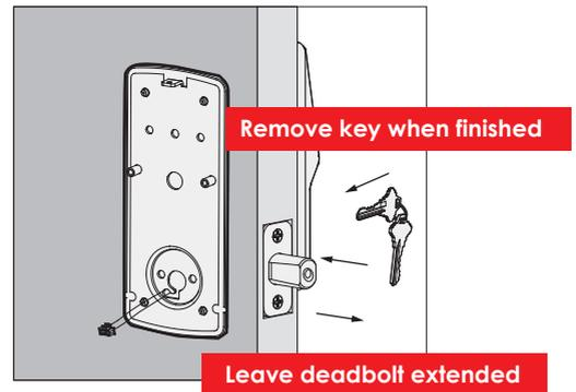
**4:** Use the key to ensure deadbolt locks and unlocks smoothly (no binding or rubbing). **IMPORTANT: when finished, leave the deadbolt extended and remove the key before proceeding to the next step.**
