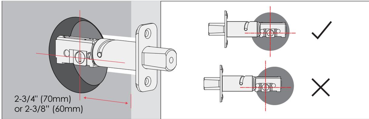
The deadbolt comes set to 2-3/4" (70mm). Adjust length to 2-3/8" (60mm) if necessary. (wear gloves to protect from possible pinching).
