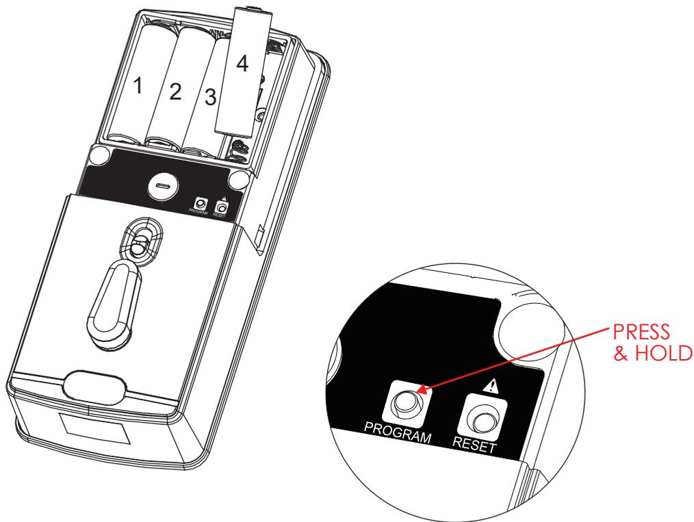
**1:** With door open and deadbolt **fully extended**, place ribbon inside compartment and **insert 3 batteries only (hold on inserting the 4th)** in bottom row (note correct -/+ polarity).
