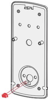
**1:** Check interior mounting plate (K) alignment to your door hole before securing with adhesive strips.
