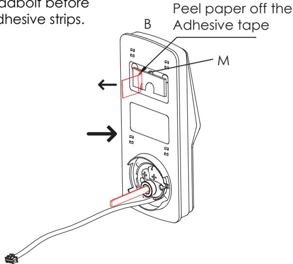
Peel film from adhesive strips and make sure torque blade is in the vertical position with the deadbolt extended. Place assembly and torque blade through the deadbolt slot and guide connection cables through the cross-bore hole under the deadbolt as shown. Complete mounting by aligning and securing until flush to exterior door surface.
