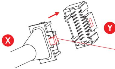
Plug **X** into **Y**, match red side of plug with red on socket - insert tightly.
