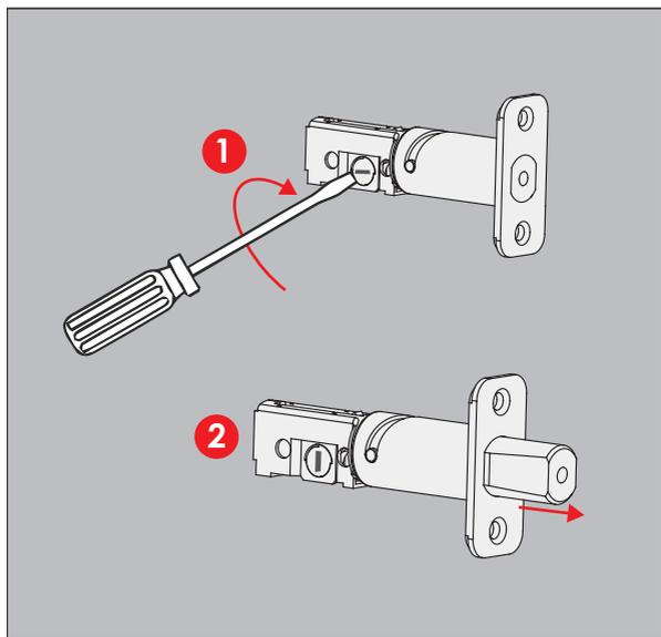
Insert the deadbolt into mortise flush with door edge, make sure that the right side is up and the slot is in the vertical position. Secure with 2 **K** screws.
