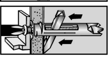
3. Push screw firmly through E-Z Toggle to engage clamp before turning screw. Turn screw. Toggle tightens against back of drywall.
