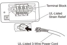
Attach the two hot leads (black and red) of the power cord to the outer terminal block screws.
