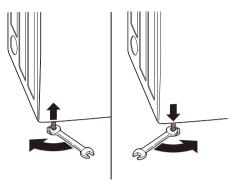
If you are installing the dryer on the optional pedestal, you must use the leveling feet on the pedestal to level the dryer. The dryer leveling feet should be fully retracted.
