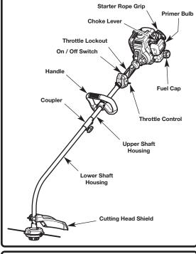
Press and hold the handle base against the underside of the upper shaft housing. Press the handle top onto the handle base until they snap together. Insert the bolts (x4) into the holes (x4). Tighten the bolts, but do not tighten them completely. Use a 5/32-inch (4 mm) Allen wrench.
