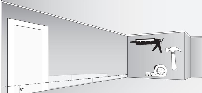
Starting on the floor, draw a level line at 6" from the floor. Next, attach the first plank in the left corner and add construction adhesive to the back of the plank then nail in place (see instructions above). Repeat this process until you reach the right wall cutting the pieces as needed. Stagger the next row of planks over the joints and cut pieces to fit as needed until you reach the ceiling. Finally add wood trim at the floor to finish your installation if desired.
