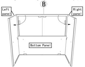
Step 2: Unfold the bottom shelf from Body (B) as below.
