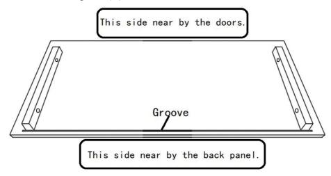
Step 5: Open the doors, attach the Tabletop (A) to the Body (B) with Hex bolts (H1) and Washers (H2) by Allen key (H4) as shown in picture below. Fully tighten all bolts.
