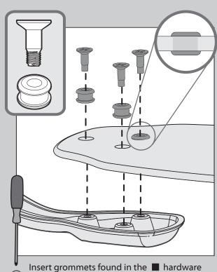
bag into the holes in the hardware bag into the holes in the blades, then secure each blade to a blade iron with screws found in the hardware bag.
