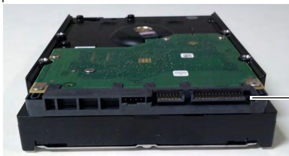
HDD power and SATA connector
