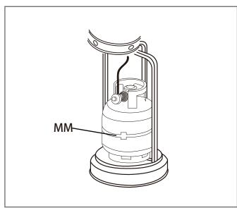
12. Turn the cylinder valve on the tank clockwise to close the propane tank. Attach the regulator (H) to the cylinder valve by turning the regulator coupling nut clockwise. Make sure it is fastened securely and tighten connections by hand only.
