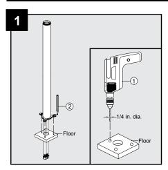
Drill a hole 2 1/4 in. diameter min. - 2 9/16 in. diameter max. in the floor with an electric drill (1). Mark the locations for the screws with a pencil (2). Then drill three holes 1/4 in. diameter for the screws in the floor with an electric drill (1).
