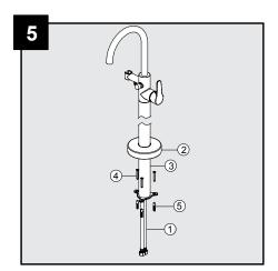
Place the assembly with the flexible supply lines (1) through the prepared hole. Then holding the escutcheon (2), secure the standpipe (3). Note: If mounting into wooden floor, secure the standpipe (3) using screws (4) only (wall plugs are not needed). If mounting into solid floor, mark the position of holes first and then secure the standpipe (3) using anchors (5) and screws (4). Where requried ensure correct anchors for your floor type are used.
