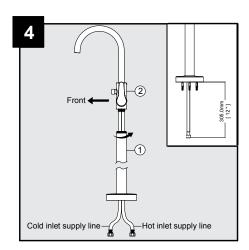
Screw the standpipe (1) onto the mixer (2) by hand. Turn in a clockwise direction until it is tight. Note 1: Do not to reverse the cold and hot supply lines. Note 2: After installing the standpipe (1), the inlet supply lines will be exposed 12 in. below the standpipe. Please pay attention to set aside enough space to connect the water supply lines and prevent the water inlet supply lines from twisting.
