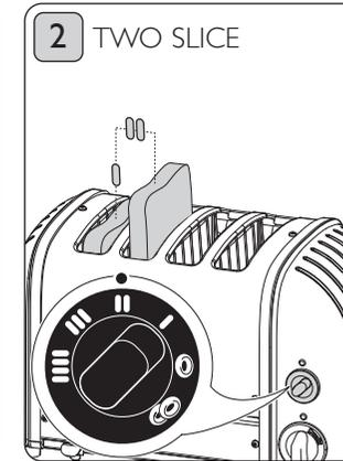
Rotate to the two slice indicator. The first two slots from the left will toast on both sides.
