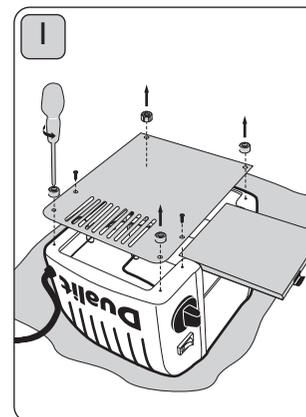
1 Unplug and place toaster on a soft cloth. Remove crumb tray and unscrew feet to remove the base plate.
