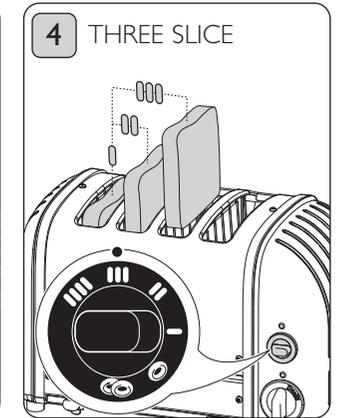
Rotate the 'selector switch' clockwise to the three slice indicator. The first three slots from the left will toast on both sides.
