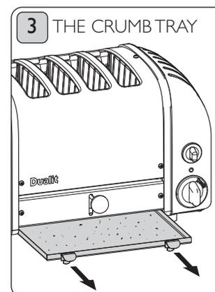
Empty the 'crumb tray' on a regular basis. Daily if being used in a commercial kitchen.
