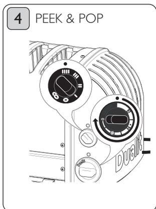
Check the progress of your toast at any time by pushing down on the 'ejector knob'.
