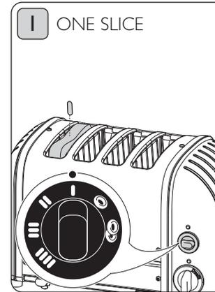
Rotate the 'selector switch' clockwise to the one slice indicator. The left hand slot will heat up on both sides.
