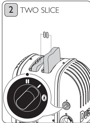
Rotate the 'selector switch' clockwise to the two slice indicator.
