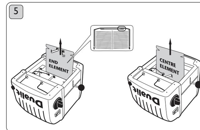
5 Remove element. To re-assemble, reverse procedure ensuring wires and parts are correctly positioned. Ensure new element is marked the same as the one removed and is seated correctly in the channels either side. PAT test before use.
