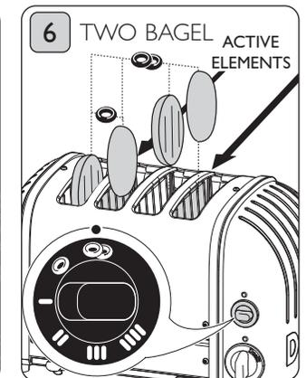
Rotate the 'selector switch' anti-clockwise to the two bagel symbol. Only the second and fourth element from the left will heat up.
