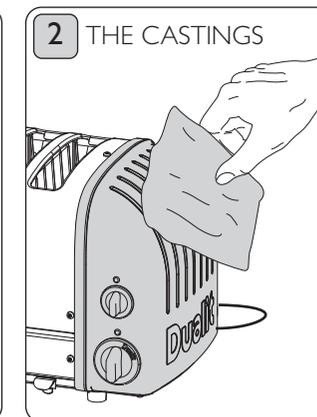
Wipe the aluminium end castings with a damp cloth. Do not use a chemical or abrasive cleaner.
