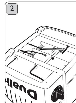
2 Loosen locking nuts on retaining plate using a 6.5mm spanner and slide back.
