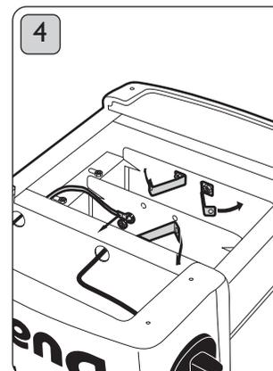
4 Bend brass links and wires away from the element.
