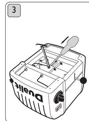
3 Unscrew brass links and wires.
