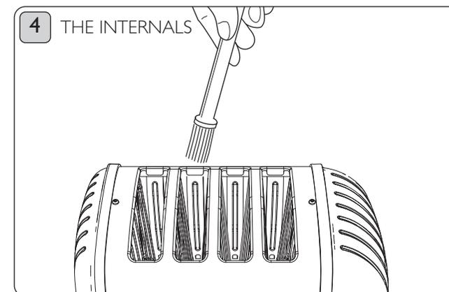
With the toaster unplugged use a **SOFT BRUSH** to clean inside your toaster; do not use a sharp or metal utensil! Crumbs should be carefully brushed off the elements using only a soft brush, the toaster can be turned upside down and excess crumbs be shaken out.
