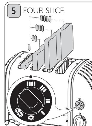
Rotate the 'selector switch' clockwise to the four slice indicator. All slots will heat up.
