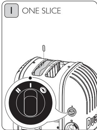
Rotate the 'selector switch' clockwise to the one slice indicator.
