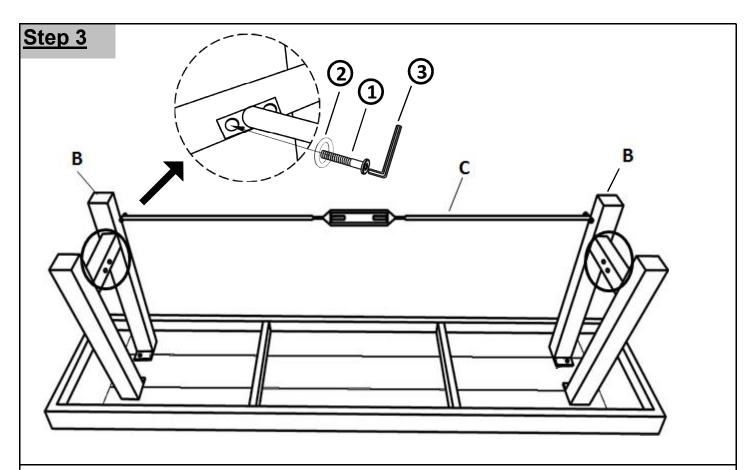
Attach the Turnbuckle Set(C) to the Iron Legs(B) using Bolt( $\widehat{1}$ ) and Washer( $\widehat{2}$ ) with Allen Key( $\widehat{3}$ ).
