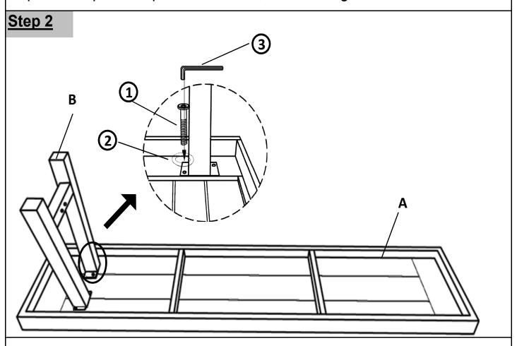
Place the Seat(A) facedown onto a clean, non-marring surface. Attach Iron Leg (B) to the Seat(A), using Bolt(1) and Washer(2) with Allen Key(3).
