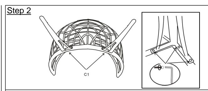
Attach two Front Legs(C1) to the Basket Seat(A) using Bolts with Washers(H) with Allen Key(G) as shown in the picture above.
