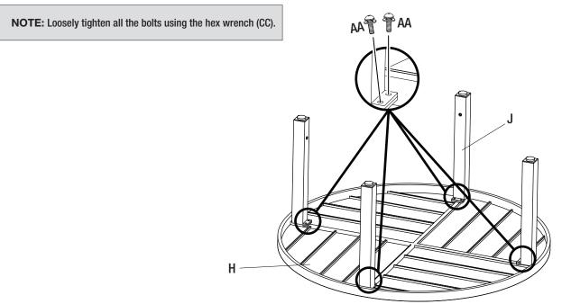
Connecting The Leg Connector To The Table Legs
