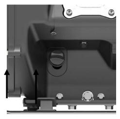
Figure 1 - Unscrew the Dipstick Cap
