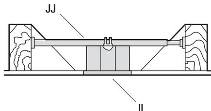
To hang your fan where there is an existing fixture but no ceiling joist, you may need an installation hanger bar (JJ) (not included) as shown above.
