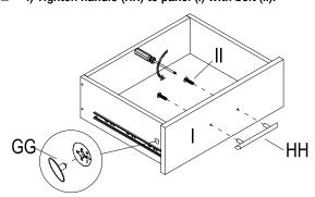
g) Cover the cam holes with the cover (GG).
