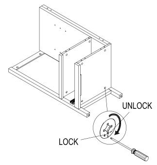
Cam lock bolt Wood dowel Cam lock Small head Large head
