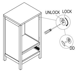
e) Cover the cam holes with the cover (DD).
