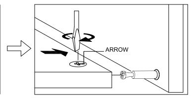
NOTE: The arrows on the hidden cam-locks should point to the cam-bolts.
