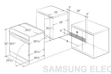
A: Cabinet opening min 30" B: Acceptable electrical outlet area
