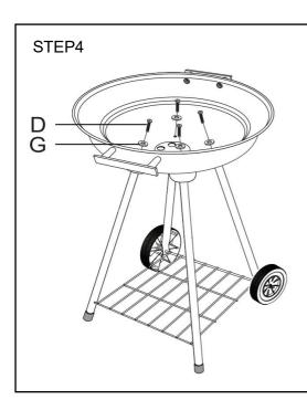
4.1 Use four screws (D) and washers (G) to lock the assembly in Step 2 and the assembly in Step 3.
