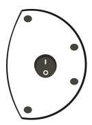
The rocker power switch on right side to control power on/off.
