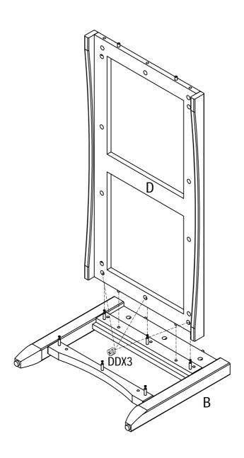
Sonnect bottom panel(F) to side panel(B) with cam lock(DD) from step 7
