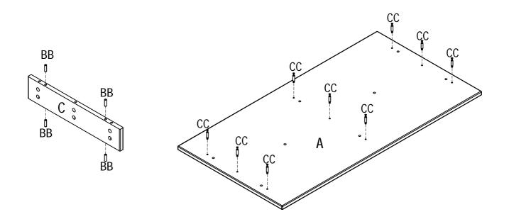
Attached wooden dowel(BB)to bottom panel(F) and layer box(D),locked cam bolt(CC) to layer box(D)
