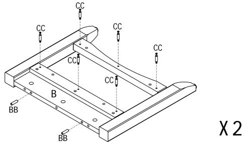
2 Lock cam bolts(CC) to the top panel(A), attached wooden dowel(BB) to divider panel(C)
