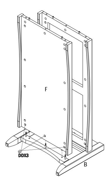
${\bf 9} \ \ {\bf Connect \ side \ panel (B) \ with \ cam \ lock (DD) \ from \ step \ 8}$
