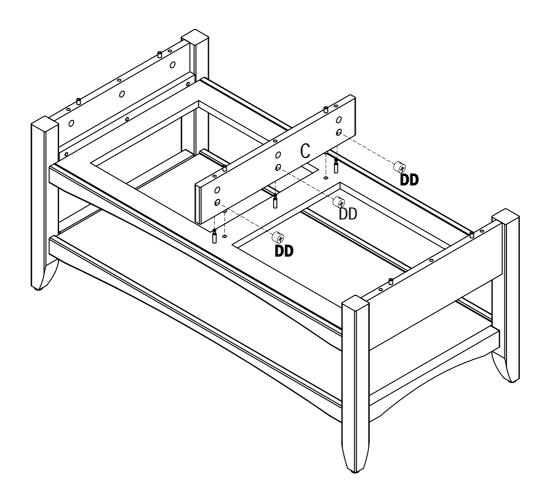
1 1 Connect table top panel(A) with cam lock(DD) from step 10
