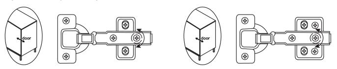
Adjust the in-and-out screws until the door is aligned with the side of the cabinet.
