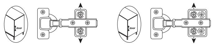
Loosen the height screws, then move the door up or down to make it level.
