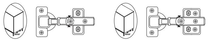
Loosen the side-to-side screws, then screw counter-clockwise to make the gap wider or clockwise to close any gaps.
