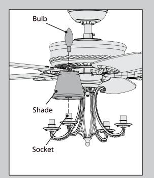
To install each shade, remove the plastic covering and place the shade over the socket so the ring in the center of the shade fits onto the socket, then install the bulb. When necessary, replace with bulbs of the same type and wattage.
