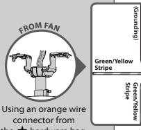
the  $\star$  hardware bag, connect the 3 grounding wires (green, green/ yellow stripe, or bare copper) coming from the ceiling, downrod, and hanging bracket.
