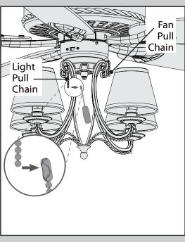
Connect the appropriate pull chain pendant to each of the short chains coming from the switch housing.
