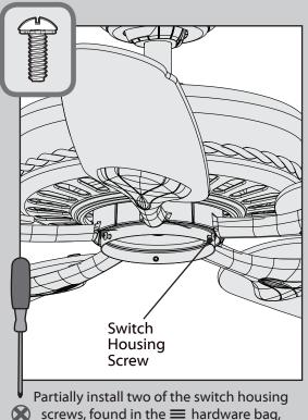
screws, found in the ≡ hardware bag, into the screw holes in the side of the upper switch housing. It does not matter which two screw holes you choose.
