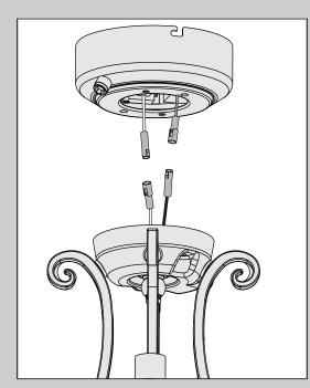
To make the connection between the light kit and the switch housing, connect the white wire from the lower switch housing to the white wire from the light kit, then connect the red wire from the lower switch housing to the black wire from the light kit.
