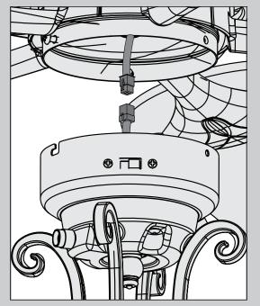
Connect the plugs from the upper and lower switch housings. Make sure to line up the colored markings on the connectors.
