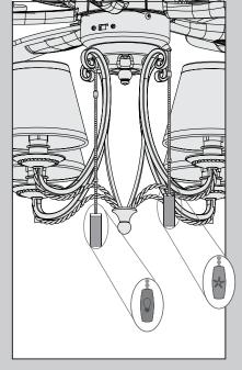
The fan pull chain controls the speed: from high to off.
