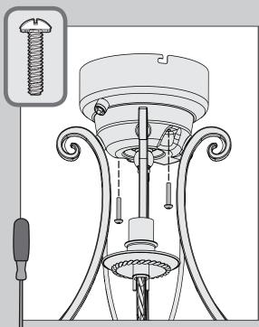
Align the screw holes in the light kit
