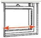
(A) Start at bottom of window. Measure distance between left and right window jamb. Add 1/4" to measurement; cut bottom fluted piece #1 to this length.
