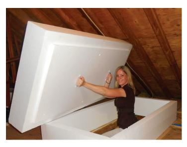
The Energy Guardian® R-38 Pull-Down Ladder Cover insulates and seals attic pull down ladders of virtually all sizes while also providing easy access to the attic for the homeowner. The unit is installed in the attic and creates a cavity for the ladder to fold into when the ladder is not in use. When assembled, the kit has the following outside dimensions: 17.75" H x 33" W x 61" L (inside dimension are 10" H x 27" W x 55" L).
