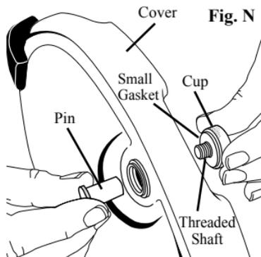
opening from the underside of the cover (Fig. N). Screw the pin portion clockwise onto the threaded shaft until it is finger-tight. Do not use a wrench to tighten the air vent/cover lock. Overtightening may cause the rubber gasket to wrinkle, which will result in the canner not sealing. When properly installed, the word (TOP) will be visible on the air vent/cover lock when viewing the outside of the cover (see Fig. J, page 16). Periodically check to make sure these two pieces are tight.
