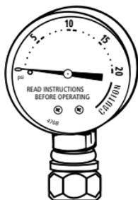
The pressure dial gauge registers pressure in pounds per square inch, or PSI. The pointer moves around the dial indicating the pressure within the unit. Pressure can be controlled and maintained by adjusting the heat setting on your stove.
