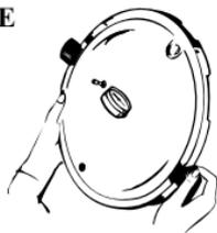
8. Check to be sure the overpressure plug is seated properly in the cover (see page 22, Fig. M).
