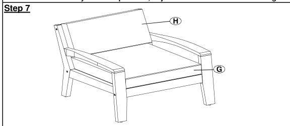
Place Seat Cushion (G), Back Cushion (H) to Seat Panel (D). Inspect it and make sure all parts are adequately connected.
