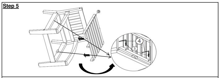
Attach the Seat Panel (D) onto the Armchair as shown in picture above.
