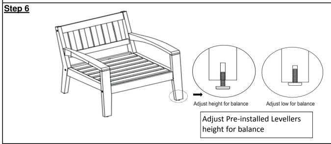
Inspect the Armchair and make sure all parts are adequately connected. In a sequential manner, tighten all Screws at all joints.
