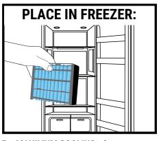
For **MAXIMUM COOLING**, place a wet filter in the freezer until frozen.
