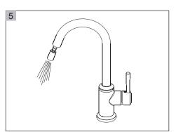
After installation is complete, remove Spray head and rotate handle to the close position. Turn Water Supply Valves on, and check all connections for leak. Flush faucet by running hot and cold water in full position for one minute.
