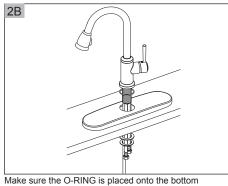
Make sure the O-RING is placed onto the bottom of Base Ring. Install faucet through Deck Plate. From underside sink, put Plastic Washer and Mounting Nut. Position faucet on sink properly and tighten Mounting Nut.
