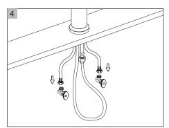
Connect hot and cold water supply lines to the Water Supply Valves.
