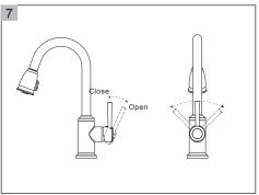
Open the valve, then turn the handle according to the sign of C and H on the handle to regulate the temperature of the water. (C=Cold,H=Hot)
