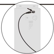
Plug the adapter into the Function Control Box.
