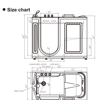
Water and electricity installation drawing
