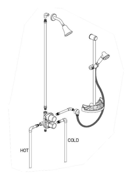
Ornellaia thermostatic valve with 2-way diverter volume control
