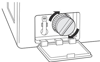
**8** Close the drain pump filter cover.
