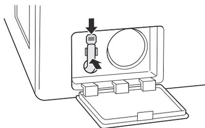
**7** Insert the drain pump filter.
