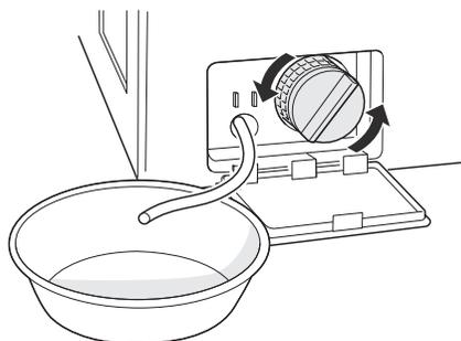
**5** Clean the pump filter and opening.
