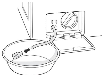
**4** Remove the pump filter.
