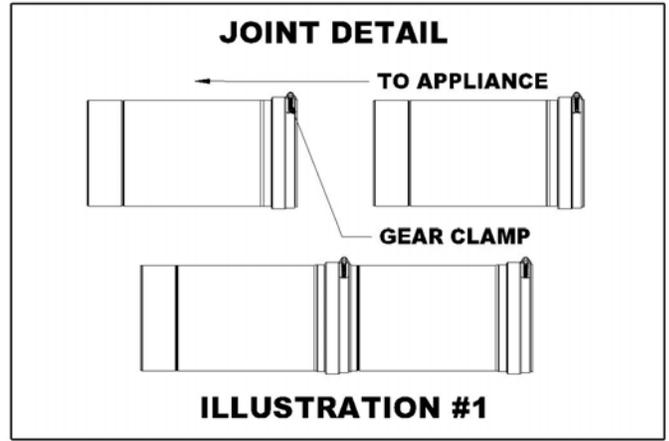
**NOTE:** Some flue collars may require the use of high temperature silicone sealant to make a positive pressure gas tight seal.
