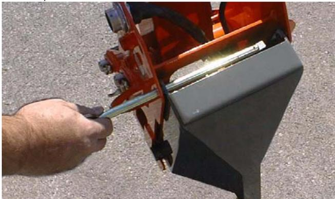
6. Remove the platform console from the platform and connect the console harness to the receptacle at the hook storage area on the turntable.
