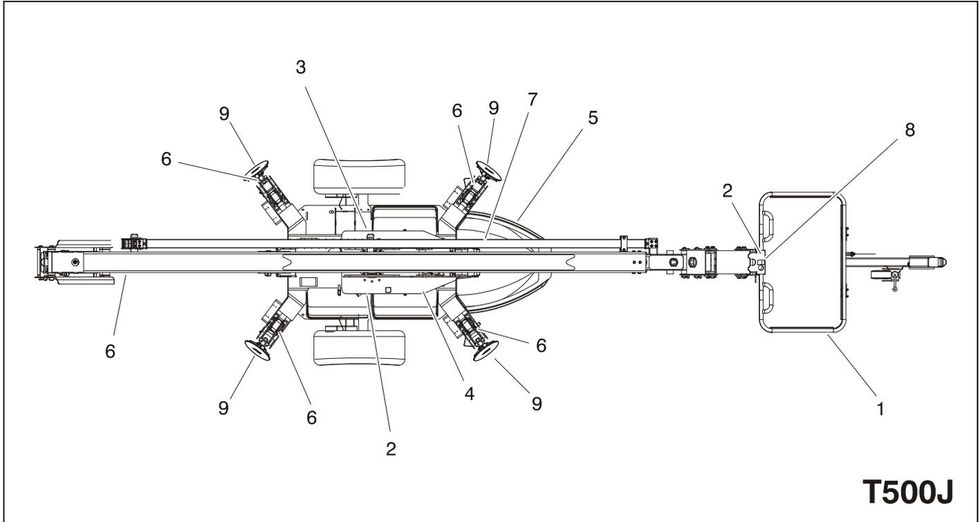
**Figure 2-3. Daily Walk-Around Inspection - Sheet 2 of 3**
