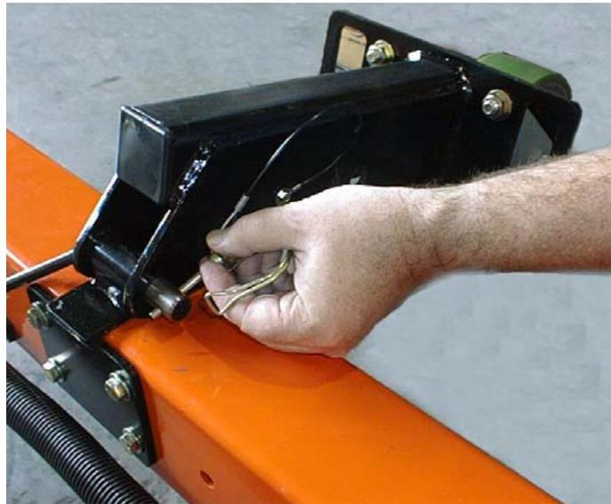
6. Pull out on the drive & set control valve knob. Ensure friction wheels are disengaged from tires.
