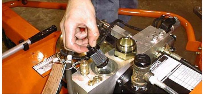
**NOTE:** The cap securing the filter must be torqued 154 to 170 ft.lbs. (209 to 230.5 Nm).
