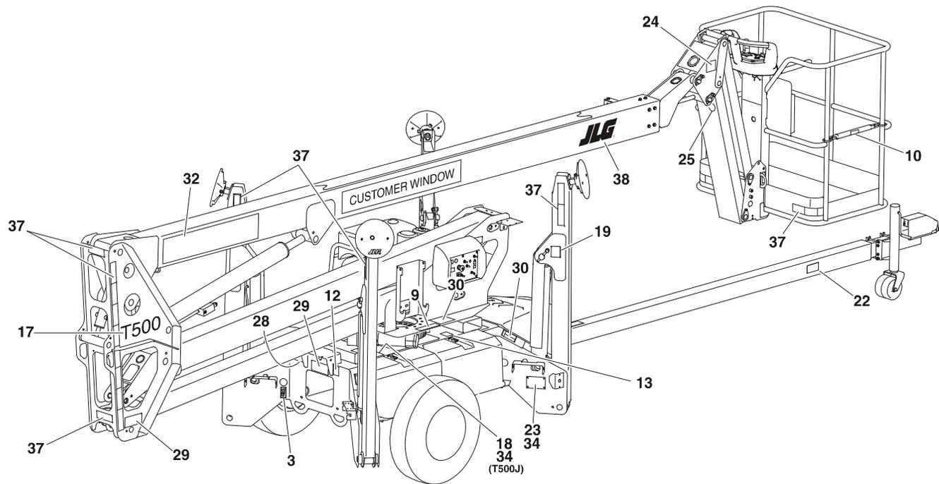
Figure 5-12. Decal Location - CE & Australia (Sheet 2 of 2)
