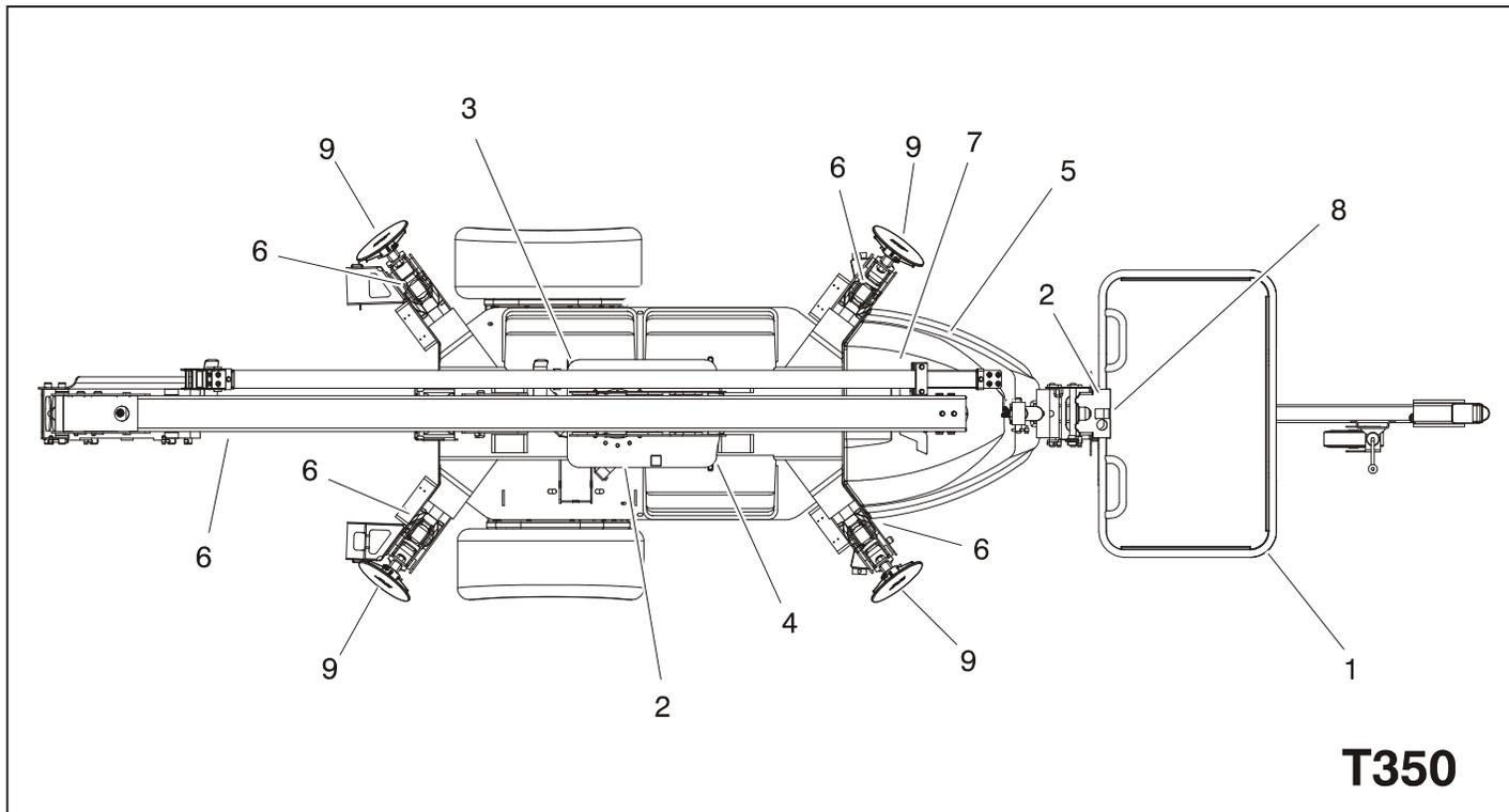
**Figure 2-2. Daily Walk-Around Inspection - Sheet 1 of 3**
