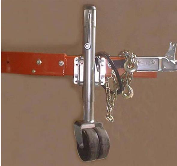
5. Remove the pin securing the jockey wheel in the drive position and swing the wheel up into the stowed position. Secure the wheel in place with the retaining pin.
