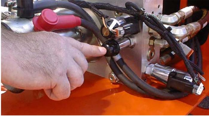
2. Locate the hand pump located on the front face of the valve block, the handle is loose mounted to the valve mounting plate.
