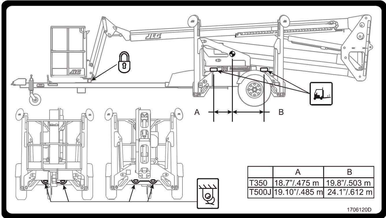
Figure 5-7. Lifting and Tie Down Chart Prior to S/N 0030000864
