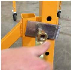
Use the Support Bracket (AA) to tighten the the Clamps (CC) and connect the outrigger to the scaffold.
