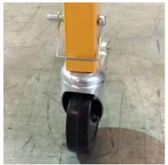
Use the Connector Pins (BB) to attach the Casters to Outrigger.
