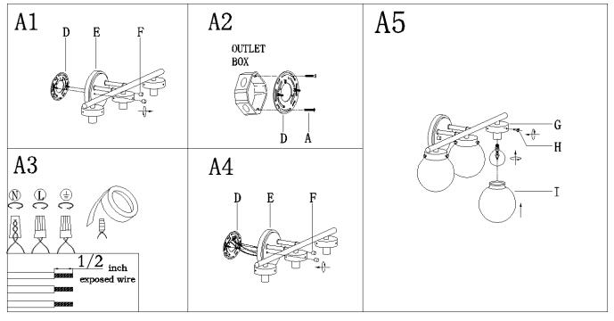
Step A1: Unscrew the studs(F) from the back plate(E) then gently remove the mounting plate (D). Step A2: Secure mounting plate (D) to outlet box with mounting screws (A). Step A3: Make wire connections
