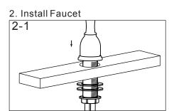
Be sure that O-Ring is placed to the bottom of the spout body. Insert Spout Shank through the center hole of sink. From underneath sink, place Plastic Washer and Metal Washer onto spout shank and tighten with Mounting Nut by hand.Before final tightening, be sure Pop-up Holefacing back.
