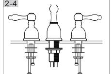
From underneath sink, tighten Mounting Nut by Tool. Before final tightening, make sure Valve Body Side Co]nnector facing Spout Body.
