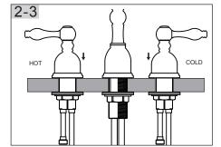
Place Mounting Nut, Metal Washer and Rubber Washer over Valve Shank. From underside sink, insert valve body through mounting holes. The hot valve, labeled with red tag should be positioned to the left side of the spout.
