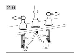
Connect Spout hot water flexible hoses to the Left Valve Side Connector. Tighten flexible hoses Nut. Connect Spout cold water supply line to the right Valve Side Connector.
