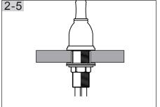
From underneath sink, tighten Mounting Nut by Hand. Before final tightening, make sure Valve Body Side Connector facing Spout Body.
