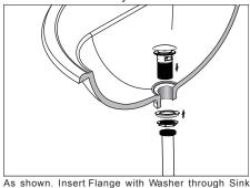
As shown insert range with washer through sink drain Hole. From underside, thread Drain Body into Flange. Holding the drain body in position with Ball Rod Opening facing back, tighten Metal Locknut securely. Thread Drain Tailpiece into Drain body.
