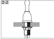
If necessary, tighten screws using a crosshead screwdriver until the faucet is firmly connected to the sink.
