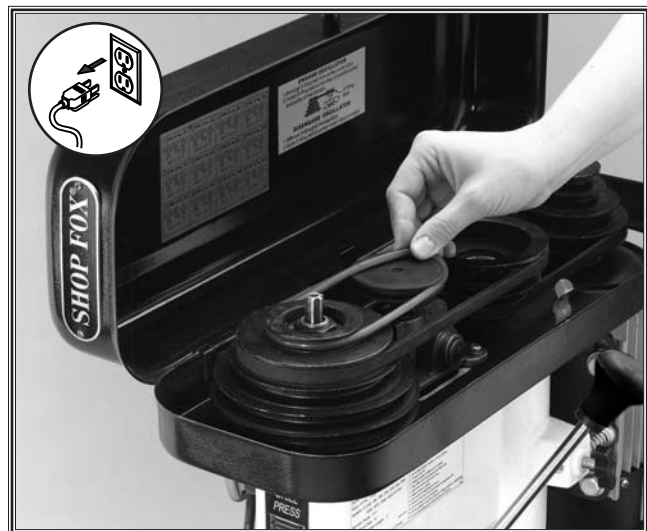
Figure 37. Stretch the belt to fit on pulleys.
