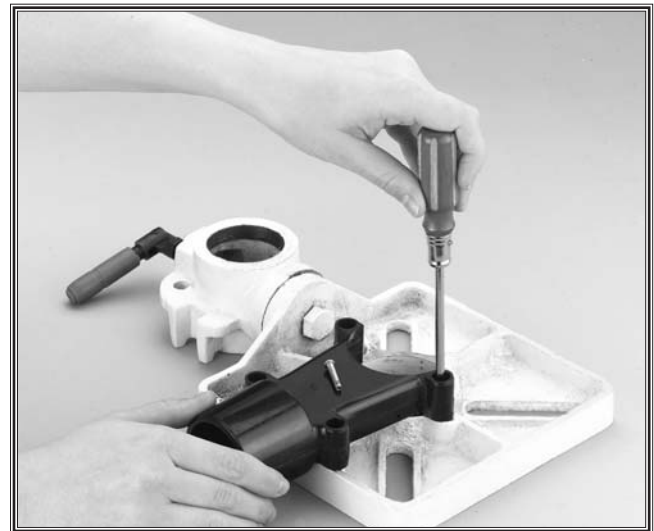
Figure 8. Installing the dust port.
