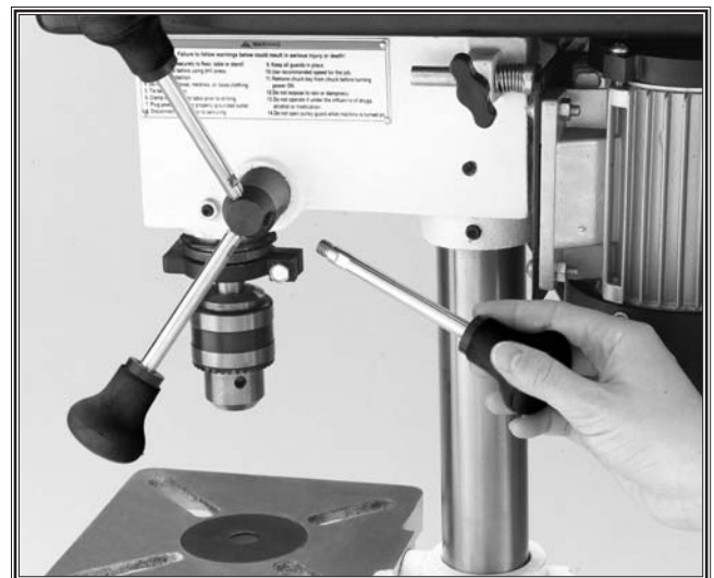
Figure 14. Installing spindle handles.
