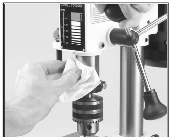
Figure 22. Clean and oil quill shaft.
