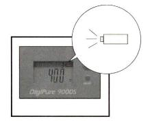
happens, replace the batteries. After the batteries are replaced, the sound and blinking will stop.
