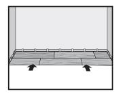
Install remaining rows, one row after the other, and maintain the required 8" (20.3cm) stagger throughout the install. Tap and square each plank as instructed in step 7.
