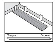
Interlock the next plank at the end joint of the first plank by inserting the tongue into the groove of the first plank.
