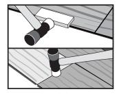
After installing the last piece of the second row, slide the entire assembly against the spacers on the starting wall, maintaining the required 1/4" (6mm) expansion space.
