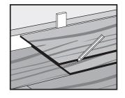
Install the plank with the cut side always facing the wall. Use a pull bar to lock the long edges together. Do not use the pull bar on the short edges.
