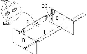
□ c) Tighten panels (B/D/G) by rotating the cam locks (AA) as shown.
