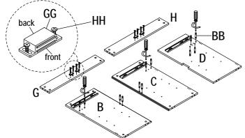
□ b)Insert wood dowels(CC) into panel(G), then connect front panels(G/I) with panels(B/D) as shown.
