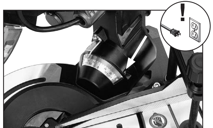
Figure 83. Bevel adjustment screws.
