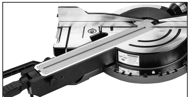
Figure 65. Finished zero-clearance insert.
