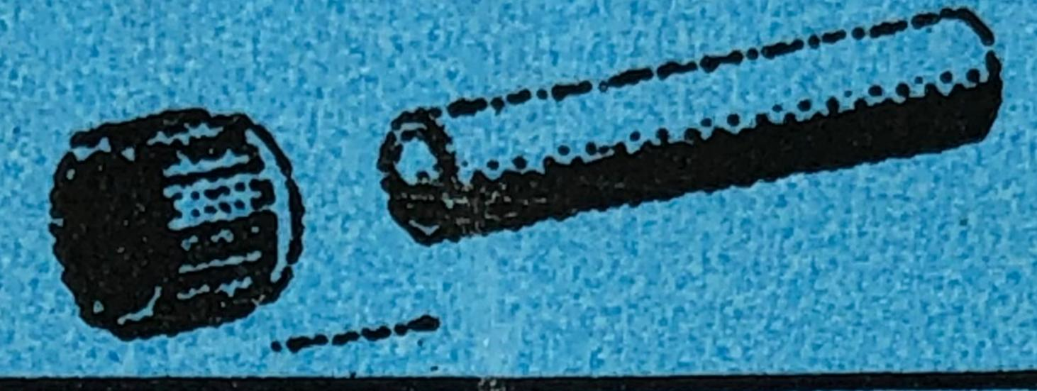
2 Firmly press tubing onto the flare of the fitting using a rocking motion until the tubing rests against the fitting.
