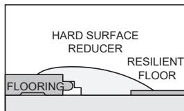
**Hard Surface Reducer:** Used to transition to another hard surface flooring of different heights such as tile, vinyl, or concrete.
