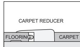
**Carpet Reducer (also called Baby Threshold or End Cap):** Used to transition floor coverings of differing heights. This reducer strip is also commonly used to border a fireplace, sliding glass door and other exterior door jambs.
