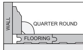
**Quarter Round:** Used to cover the expansion space between the wall base and your flooring. It can also be used to make smooth transitions between the floor and cabinetry. It can be used with or without wall base molding.
