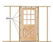
Solution: Add shims to create a square fit using levels and accurate measurements.
