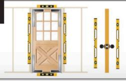
Check: Do a dry fit before installing to check all elements are fit. Once installed, double check all elements of the installed door are perfectly level, plumb and square to make a TRUEly perfect fit.
