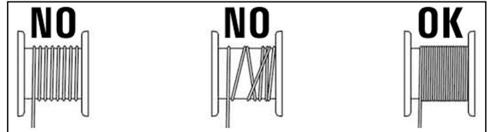
Figure 6 Make sure the cable is wound properly on the reel.
