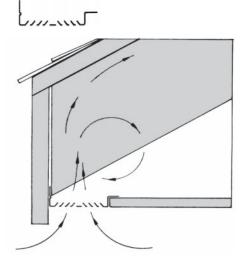
Continuous Soffit Vent always installs correctly, since arrangement of louvers is same from either side. Intake airflow from each side meets above vent to create gentle turbulence assisting fallout of snow and rain before it is carried to insulation.
