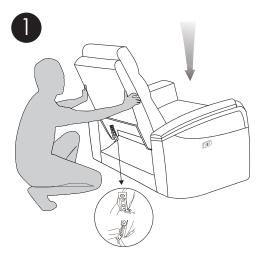
Align seat back and metal post connectors lock and slide into place.
