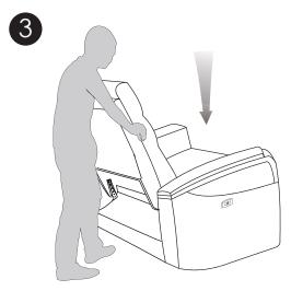
Push down firmly on seat back to lock connector
