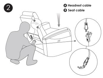
Connect the cable A into cable B.
