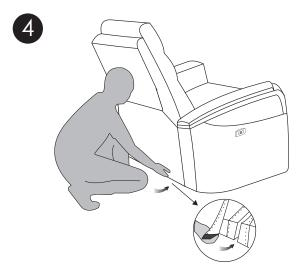
Affix back cover to bottom of the frame using the built-in hook and loop fastener strip.
